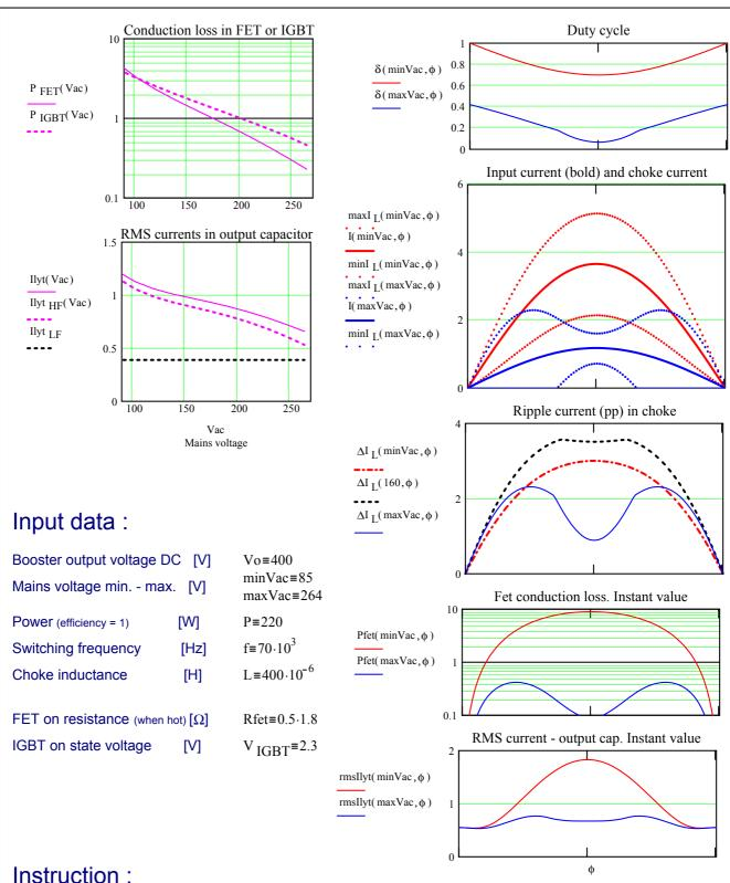
The plots in the right side show various data during one half period of the mains voltage - i.e. 10msec or 8.3msec. The zero crossings of the mains voltage are in the left and the right edge of the plots.  $\phi$  is the mains phase angle :  $\, \varphi = \, \omega \cdot t = 2 \cdot \pi \cdot f_{\, net} \cdot t \,$  .
